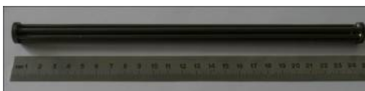
Figure 18: Hollow fibre bundle with a length of 250 mm joined by RAB method.
