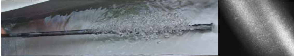
Figure 22: Bubble test of a defective membrane tube after long term test and a detail view on an axial crack.
