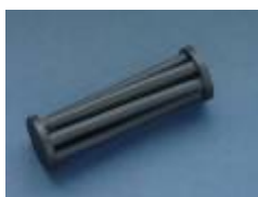
Figure 17: Hollow fibre bundle with a length of 50 mm, joined by DDR method.
